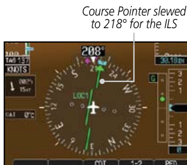
Figure 2-33 Auto-Slewing HSI with ILS Loaded and Shown with the Corresponding Approach Plate
